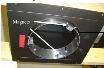
**E4.** Loosen the screws on the A2 access panel and lower the collar to be flush with FINISH CEILING drywall or flush to whatever ceiling materials are used. Be sure to use a straight edge to level the collar to be flush and parallel to the FINISH CEILING. Tighten screws securely but not too tight to pull the ring out of round or cover may not fit.
